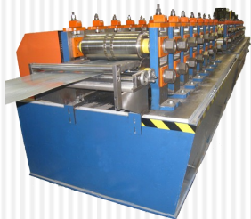
Floor decking line
