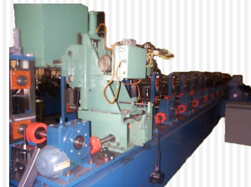
Welded Storage step beam line
